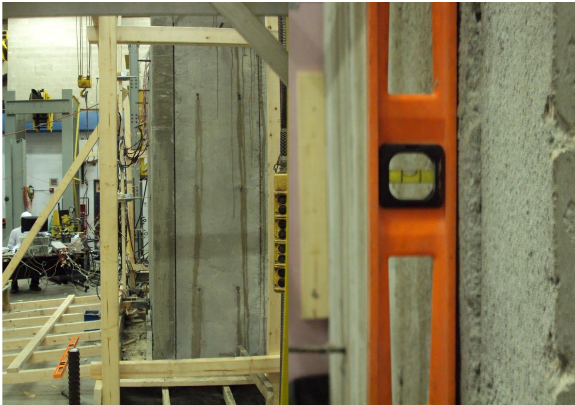
Figure 4.27: Final undamaged state of the abutment after loading.
