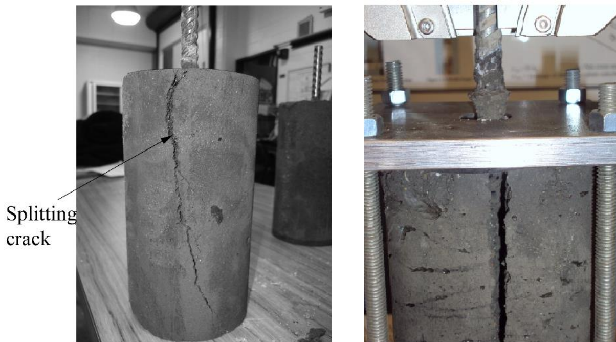
Figure 3.22: Splitting bond failure and cracks in pullout test using cylindrical specimens.
