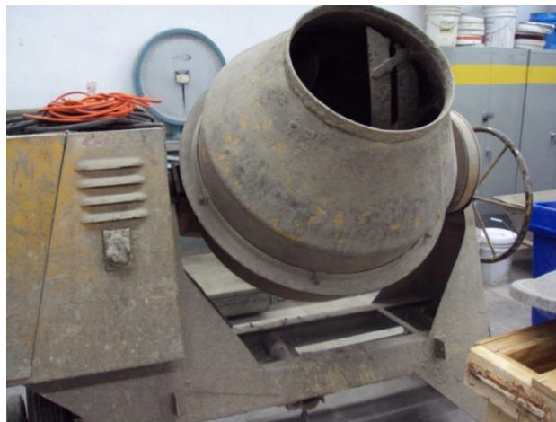
Figure 3.6: Concrete mixer used for mixing CLSM samples.
