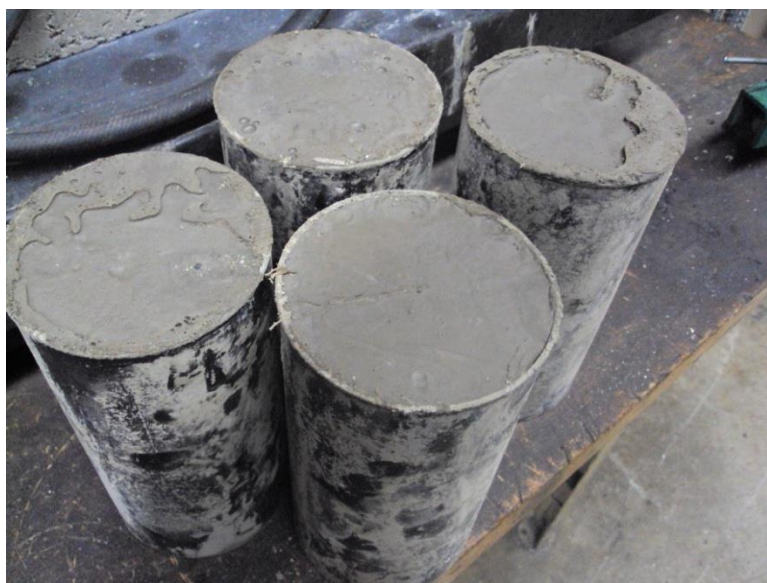
Figure 3.31: Collected samples from inside of the CLSM fill.
