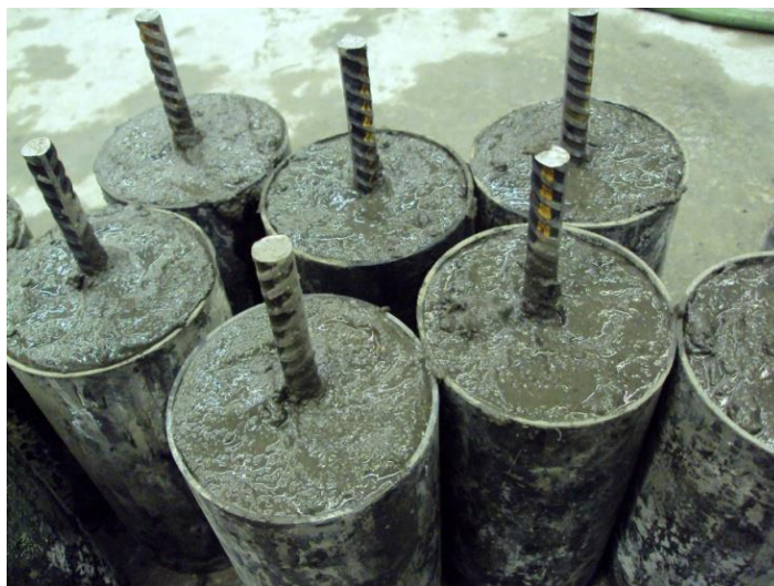
Figure 3.17: Cylindrical specimens for pullout test.
