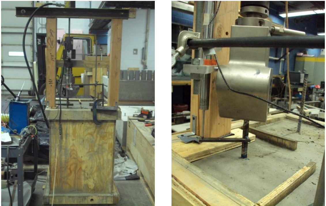
Figure 3.28: Large-scale pullout testing.
