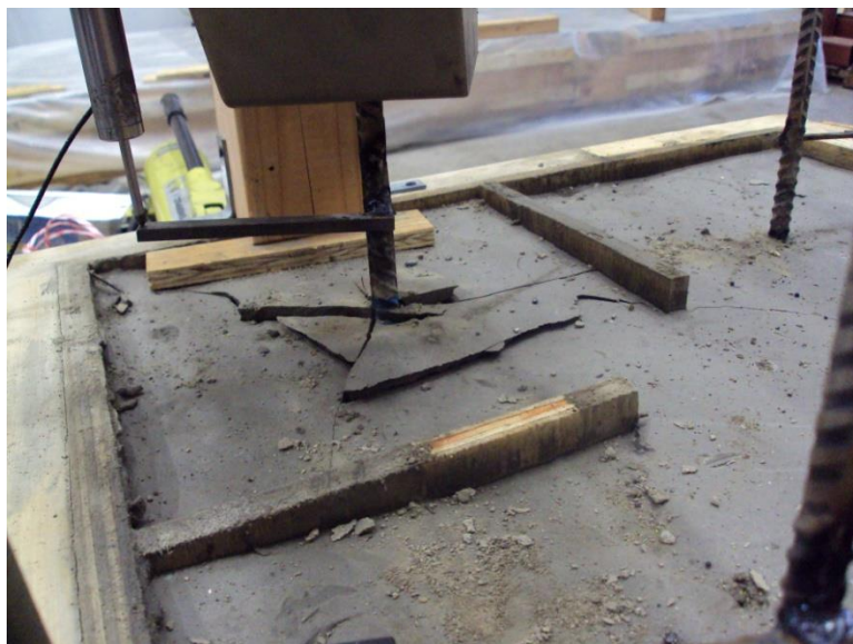
Figure 3.30: Pullout failure of rebar from CLSM (large-scale pullout test).
