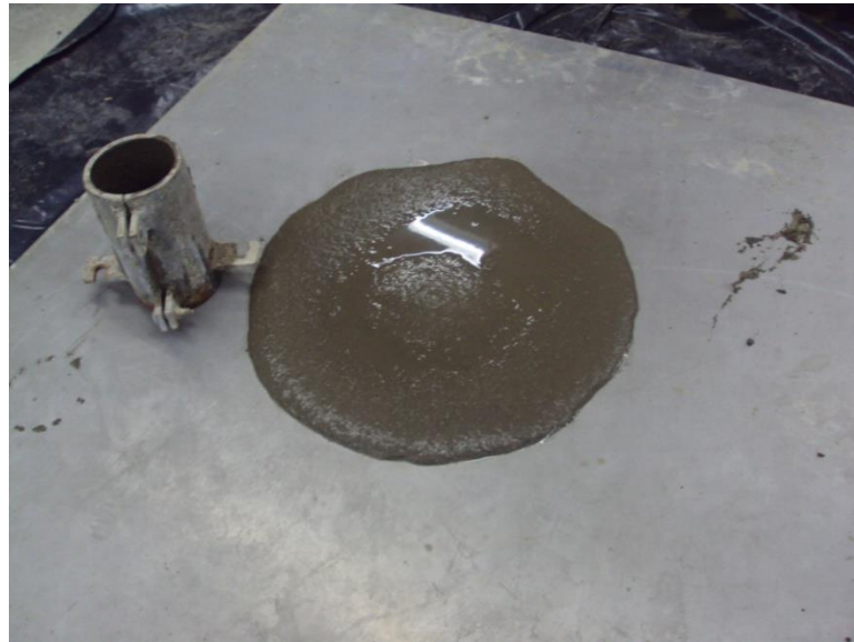
Figure 3.8: Flow cylinder test.
